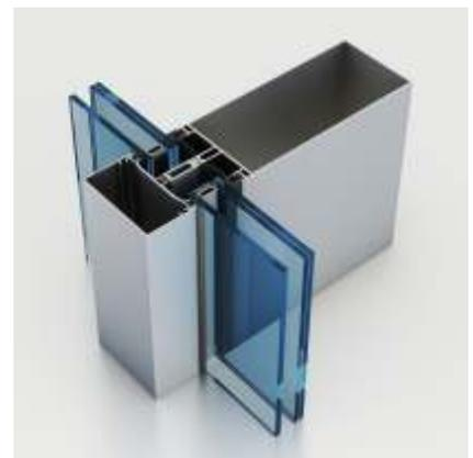
shorter horizontal extrusions span between the vertical mullions, creating a rectangular frame that binds the glass on all four sides.
